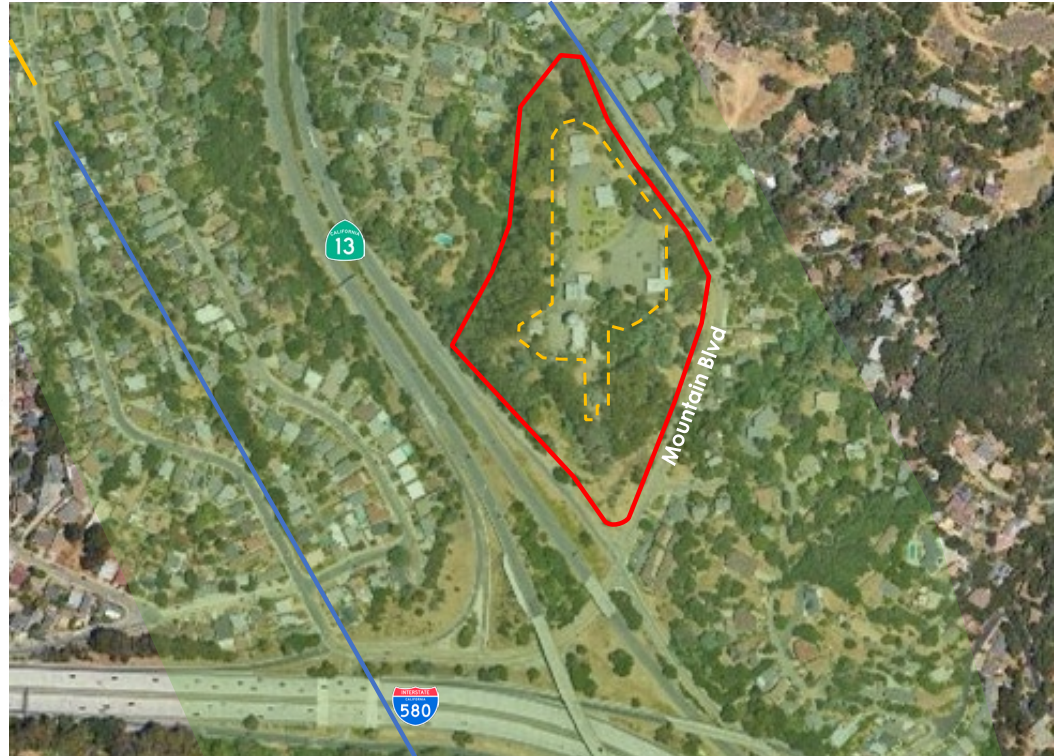
— Subject Site □ Alquist-Priolo Fault Hazard Zone — Inferred Fault Line - - - Approx. Fault Line
