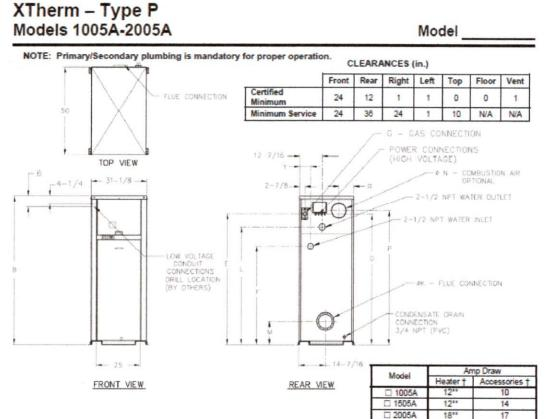
† Separate power connections are factory supplied and separate supply breakers must be field supplied. " Current draw is for heater only (Supply breaker must have delayed trip).
