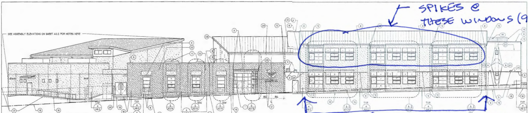
1 40TH AVENUE EXTERIOR ELEVATION SCALE: 1/8" = 1'-0" NOTE: ASSEMBLY SHOWN OBLIQUE. FOR STRAIGHT ON ELEVATIONS OF ASSEMBLY AREA SEE A3.2. NOTE: FOR FINISHING, SEE LANDSCAPE DRAWINGS
